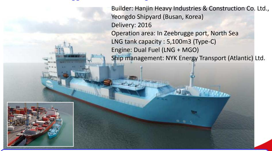
**World's First LNG Bunkering Vessel**
