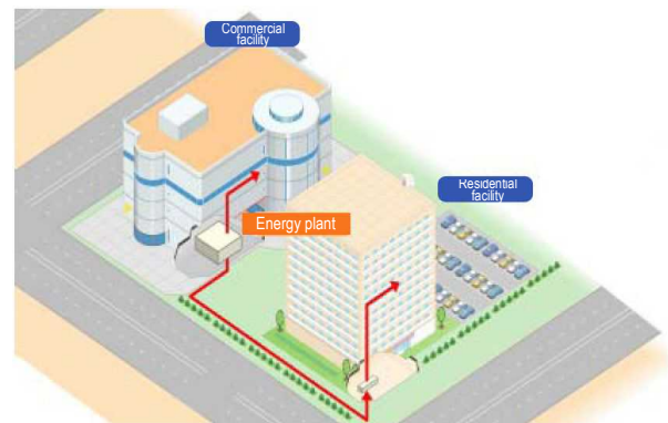
Figure 11 Point heating/cooling systems
