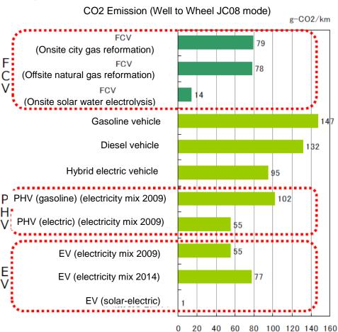
Figure 15 Comparison of CO<sub>2</sub> Emissions by Type of Vehicle, Japan CO<sub>2</sub> Emission (Well to Wheel ICO8 mode)
