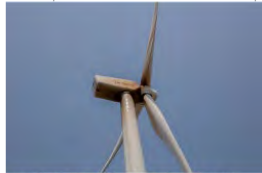
Copper-colored lubricant is seen on an Arizona SA wind turbine. Photographer: Karl Marlow/Bloomberg
