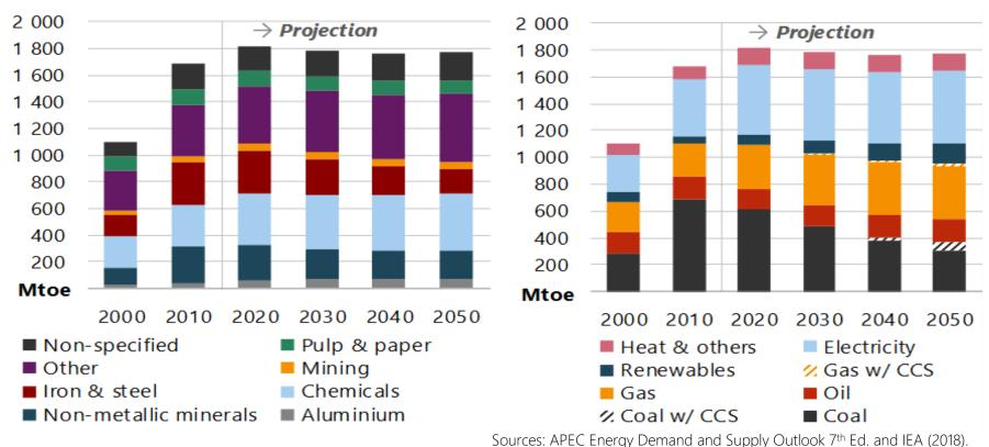
Chemical and petrochemical has the largest industry subsector energy demand; CO<sub>2</sub> emissions reduction is driven by deploying BATs, improving material efficiency, and adopting CCS technologies.
