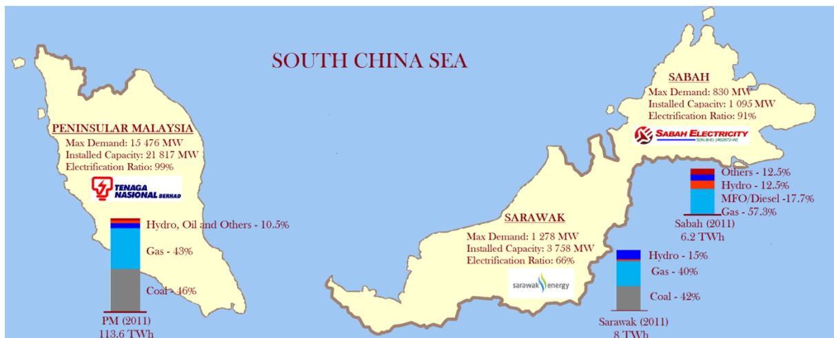
Figure 7-1: Malaysia Power Grid Characteristics
