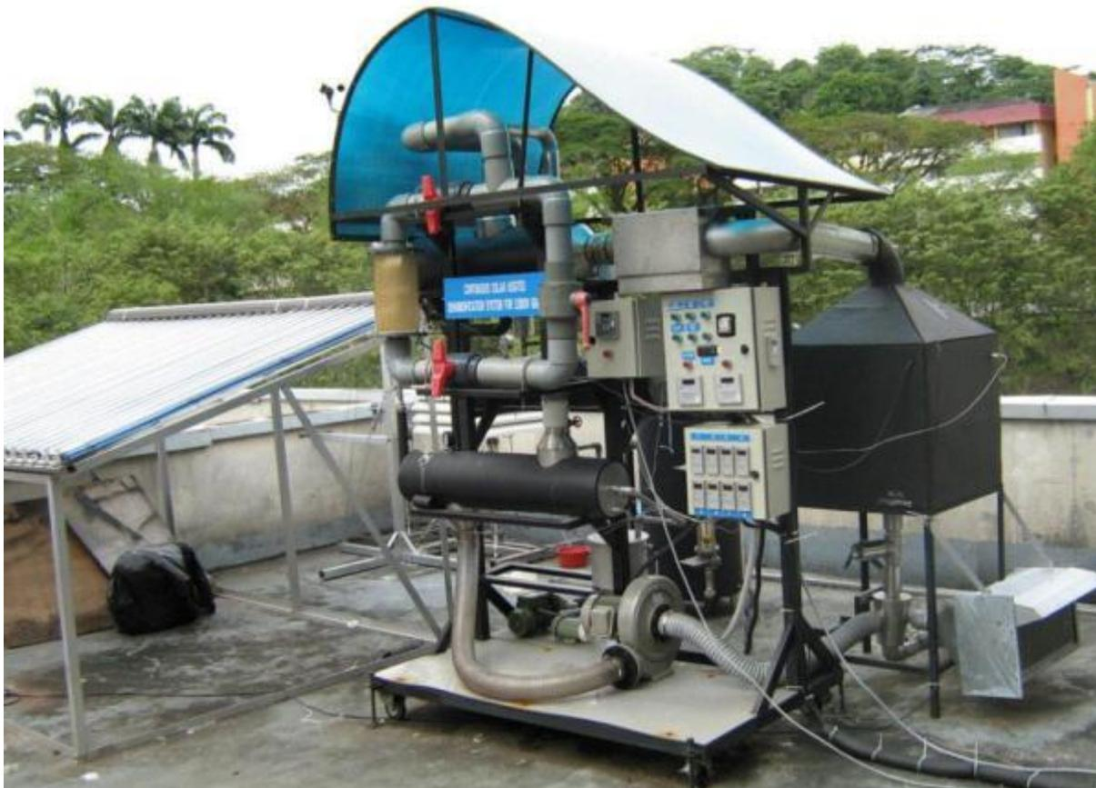
**Figure 6-9: Solar dryer with chemical heat pump (for lemongrass)**
